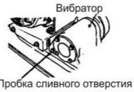
Fig-17 Vibrator Oil Plug
